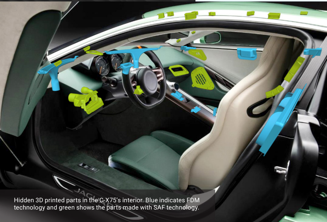
This schematic shows the 3D printed parts used in the interior. FDM technology parts are blue, SAF technology parts are green.
