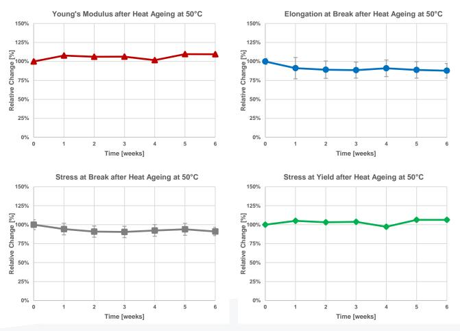
Test parameters: ASTM D638: Type IV, Pull speed: 50 mm/min, Young's modulus measured at 0.1-1.0% (regression), 22°C
