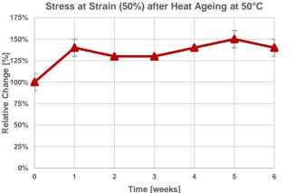
Test parameters: ASTM D412: Type Die C, Pull speed: 500 mm/min, 22°C
