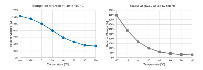
Test parameters: ASTM D412: Type Die C, Pull speed: 500 mm/min
