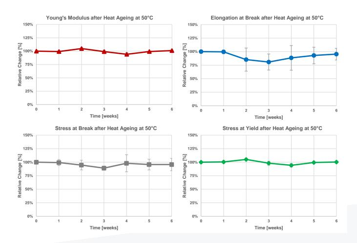
ASTM D638: Type IV, Pull speed: 50 mm/min, Young's modulus measured at 0.1-1.0% (regression), 22°C
