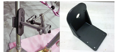
Custom tooling brackets by Orbital ATK designed for flexibility and rapid response to project requirements. FDM Nylon 12CF provides the necessary strength and stiffness.
